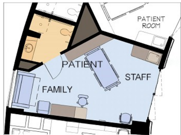
FIGURE 1: Basic universal bed / acuity-adaptable room design. The schematic shows patient, staff, and family space. Rendering courtesy of The Ohio State University Medical Center, Columbus, OH; DesignGroup, Columbus, OH; and Hammel, Green, and Abrahamson, Inc. Minneapolis, MN.
